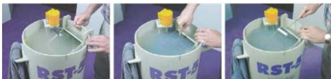
RST-5 Cleaning Station, here in use removing blue gel coat. Note: Heater & Scrubbing Board.
